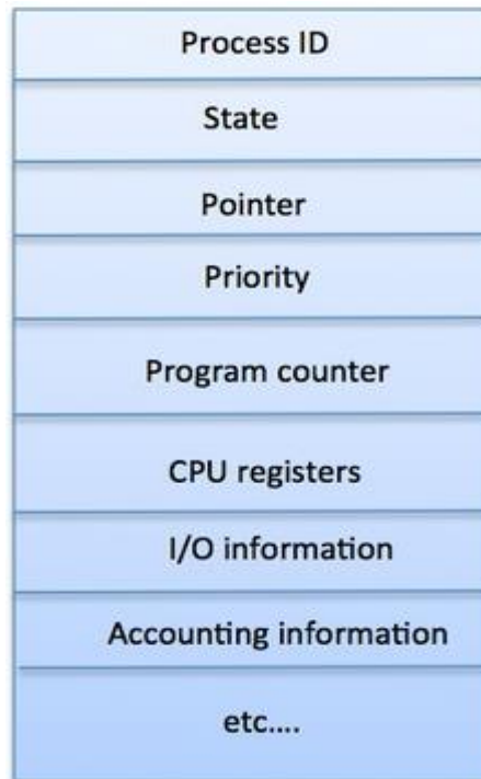
Gambar 8. Alur Block Kontrol Proses
