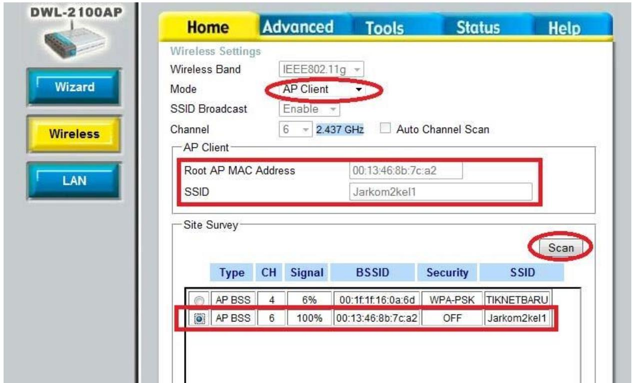
The screenshot shows the configuration page for the DWL-2100AP. The 'Advanced' tab is selected. Under 'Wireless Settings', the 'Wireless Band' is IEEE802.11g, 'Mode' is AP Client, 'SSID Broadcast' is Enable, and 'Channel' is 6 (2.437 GHz). The 'AP Client' section shows the 'Root AP MAC Address' as 00:13:46:8b:7c:a2 and the 'SSID' as Jarkom2kel1. The 'Site Survey' section has a 'Scan' button and a table of detected APs.
